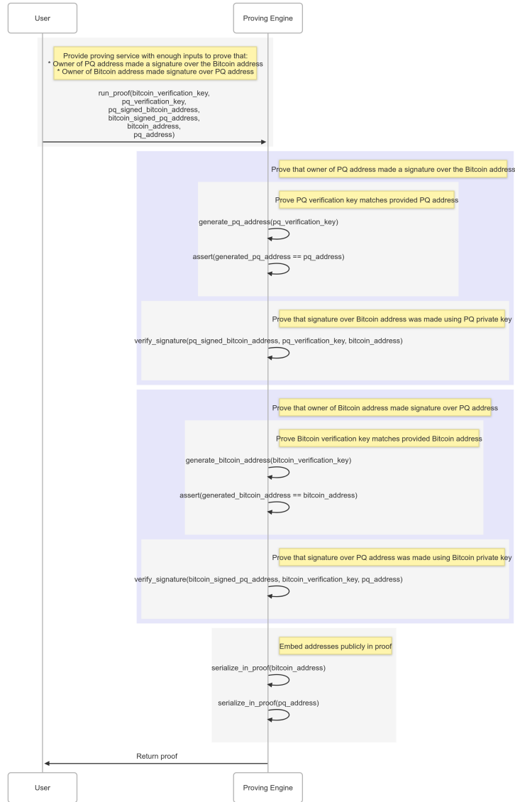
Figure 3: In-depth process of the Proving Engine’s validation steps, demonstrating rigorous cryptographic verification and the creation of a publicly verifiable proof embedding both addresses securely.
